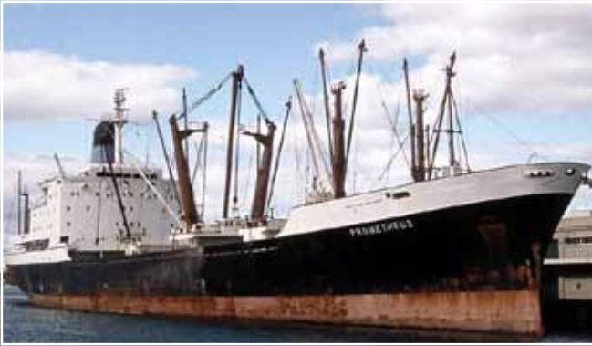
▲ The 1967-built Prometheus (12,094grt) was powered by Burmeister & Wain engines driving a single screw, which gave her a speed of 21 knots. She was sold in 1979 to C.Y.Tung of Hong Kong and renamed Oriental Merchant. Although she was converted into a cellular containership in 1980, her demise came as soon in March 1986, when she was sold for breaking at Kaohsiung.
